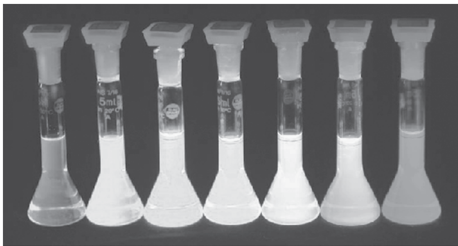
FIGURE 1: These flasks contain suspensions of nanosize CdSe particles known as “quantum dots.” The color arises after UV illumination. The only difference between the flasks are the size of the particles, ranging from 2 nm (left) to approximately 5 nm (right).
