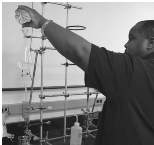
Demonstration of a column experiment during the design of Lesson 4 (Bacterial Transport). The sand column simulates sediment, while fluorescent beads are used to simulate the passage of bacteria. Dr. André Green is shown performing the experiment.
