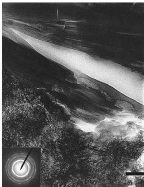
FIGURE 2: Other more powerful techniques such as Transmission Electron Microscopy (TEM) reveal the true story of the sediment at the nanoscale. Here the black scale bar in the lower right corner is 100 nm. The box inset to the lower left is a diffraction pattern, used to identify minerals. The results of this study helped identify which nanoscale minerals were serving as hosts to carry toxic metals downstream. For example, clay minerals dominate the center and top, while <10 nm grains of the iron oxide mineral hematite dominate the bottom.
