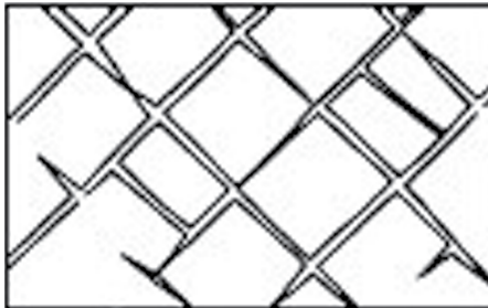
FIGURE 5: Fractures in rocks are depicted. Depending on the width of the fracture openings, bacteria can either be transported with water or they may be strained.
