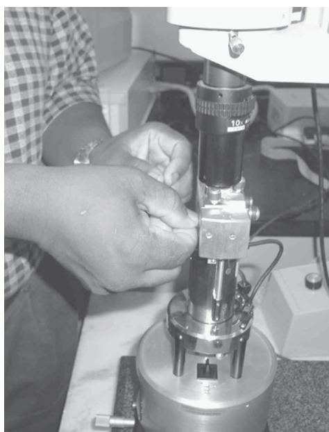
Side view of a scientist loading an atomic force microscope (AFM), a major tool in nanotechnology.
