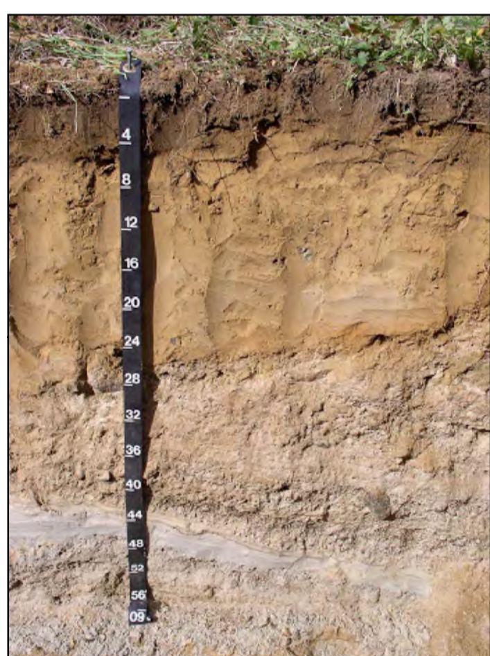
Enfield soil formed in stratified sand and gravel outwash with a silt loam windblown loess surface. The finer materials at the surface make this a prime farmland soil.
